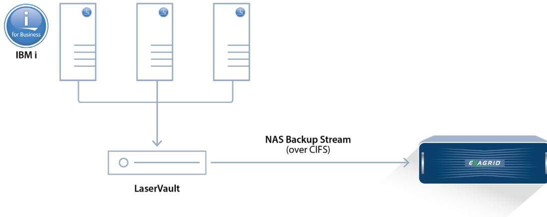
To back up data from an IBM iSeries, simply use LaserVault Backup with an IP network connection to the ExaGrid appliance and configure the LaserVault backup jobs to use a CIFS mount. The result is that backups from the iSeries are written to a virtual file on the ExaGrid which can then be deduplicated and replicated. The backup files are available at any time for rapid restore. This eliminates the need for a tape drive/library, complex VTLs, and expensive licensing found in many other products.
